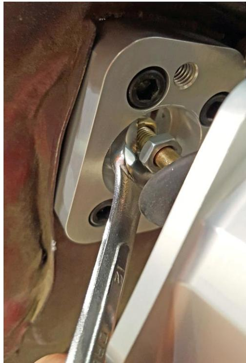
Silver nut used for adjusting 1.4" gap. Gold nut gets tightened once gap is set.
