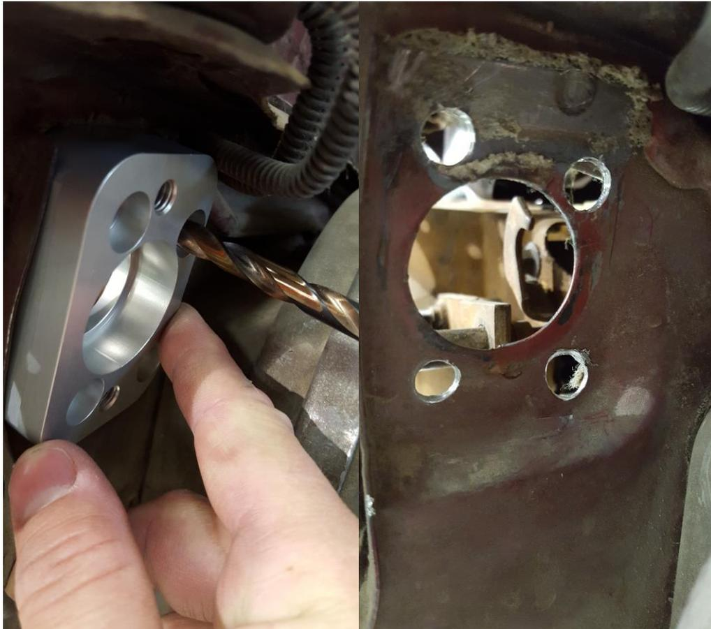
Shown are the outer firewall block "registered" on large hole & held with fasteners, then the four drilled holes.
