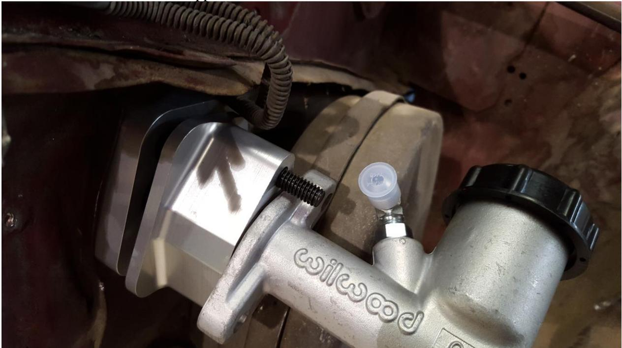
2.10 Pull out the master cylinder and rotate. Align and install nut on stud, and install lock washer and bolt in lower hole.
