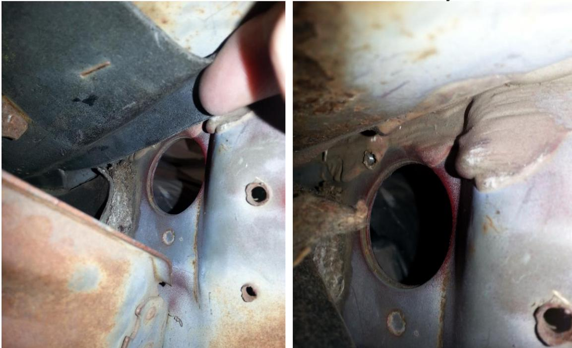
Shown are the insulation liner and excess sealant removed.
