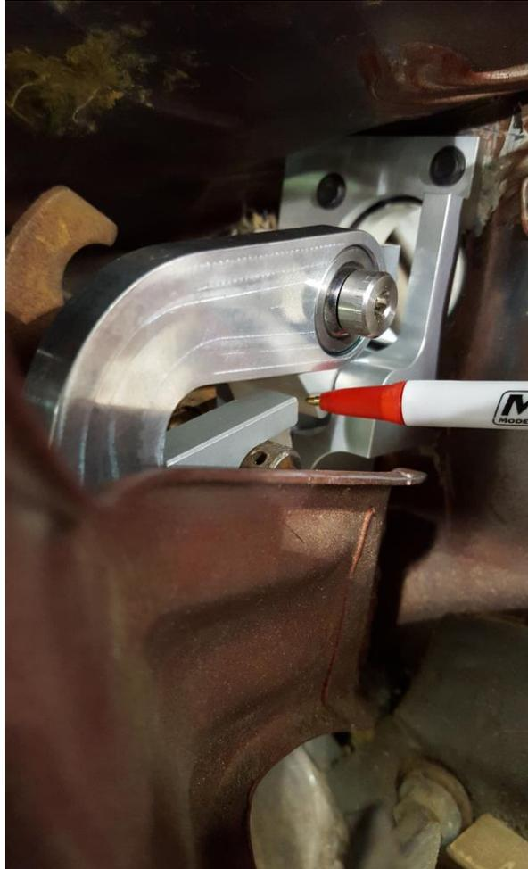
2.6 Align the Clutch Plate to be parallel with the inner edge of the Custom Clevis and tighten the set-screws in the Clutch Plate. Push the clutch pedal all the way down to tighten the rear set screw and all the way up to tighten the forward set screw. It is important the Push Lever be as straight as possible. **Do not scale the location of the Clutch Pedal Plate on the pins. Each car may be slightly different.**
