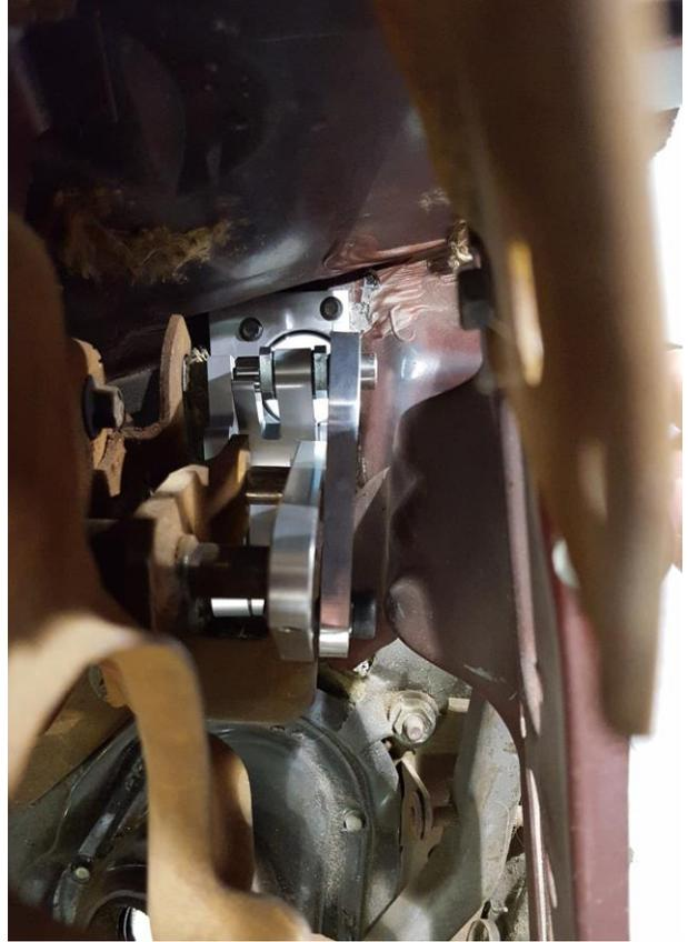
Shown is clutch pedal down, tightening set-screw and a slight gap between the Push Lever and the Clutch Plate.
