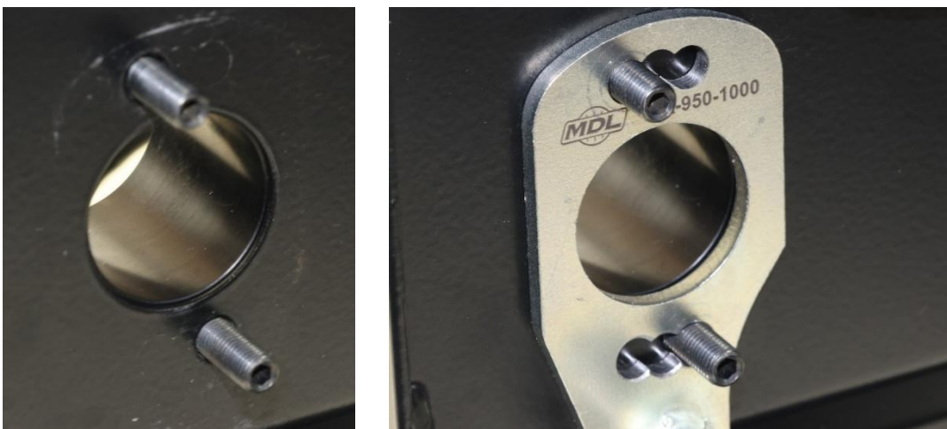
Drilled position shown for use with a brake booster for master cylinder clearance.
