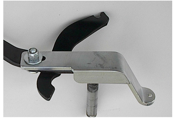
(The bracket shoulder should be against the clutch pedal).
