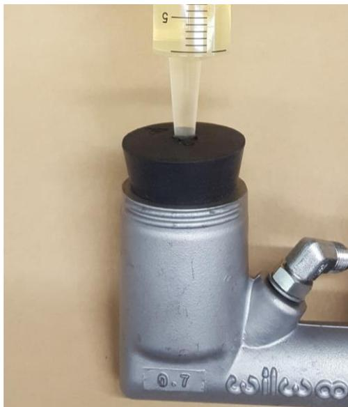
Shown is the beaker stopper pressed firmly in the opening and syringe tip in beaker stopper.
