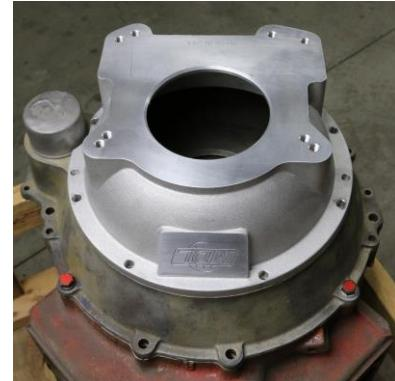
2.3 If the adapter doesn't sit flush, there may be slight interferences that can be removed with a file, or sanding disk.
