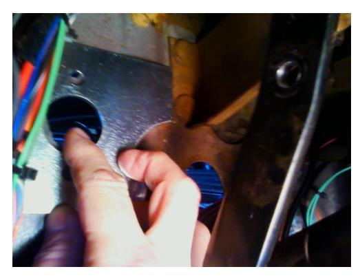
2.3 Clean surfaces of supplied plate, firewall and clutch master cylinder. Apply a thin layer of silicone sealant around edges of body plug, plate and clutch master cylinder. Install clutch master cylinder and plate using 5/16 x 1-1/4" bolts and lock nuts. Install body plug in old clutch rod hole as required. Our mock-up vehicle used this location for auxiliary components.
