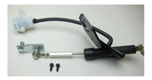
Modern DriveLine offers a complete line of **Vehicle Specific** Hydraulic Kits and we're adding more all the time.
