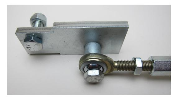
3.5 Temporarily install clutch master cylinder with plate and tighten all fasteners. Fluid reservoir may be removed to facilitate installation; protect opening from debris as req'd.
