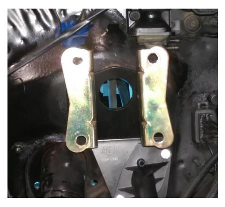
3.6 There is no adjustment on the rod/ladder joint, this has been put together with loc-tite. Install hardware thru rod end and clutch pedal bracket and tighten. Make sure there are atleast 5 full threads penetrating the rod end.
