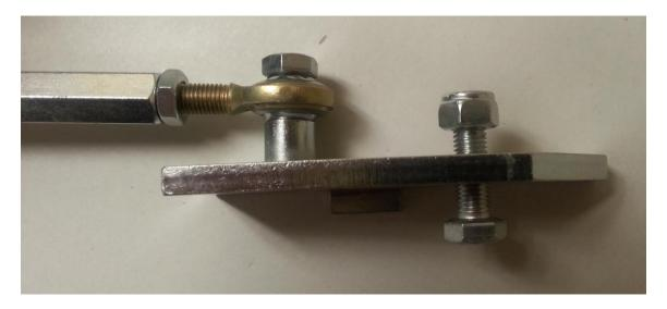
3.5 Temporarily install clutch master cylinder with plate and tighten all fasteners. Fluid reservoir may be removed to facilitate installation; protect opening from debris as req'd.
