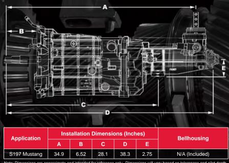
Note: Dimensions are approximate and intended for reference only. Dimensions will vary based on tolerences and pilot depth.
