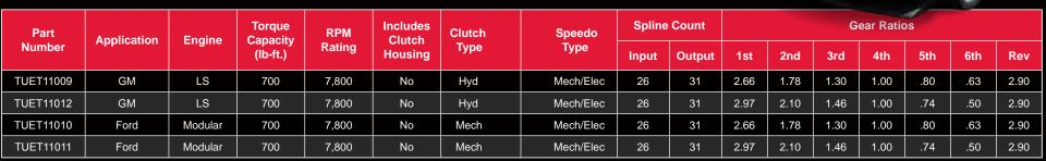
NOTE: Torque and RPM ratings may vary based on vehicle use, drivleline configuration, and quality of product installation.
