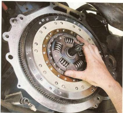
The new block plate and flywheel are installed. The Kevlar clutch disc is shown being supported with a clutch-alignment tool.
