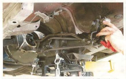
The OE transmission is lowered out of the car. The transmission jack will come in even more handy when it's time to install the new gearbox. Next, the bellhousing, pressure plate, and flywheel were removed. We also pulled the old pilot bushing out of the crankshaft using a puller specifically designed for that purpose.
