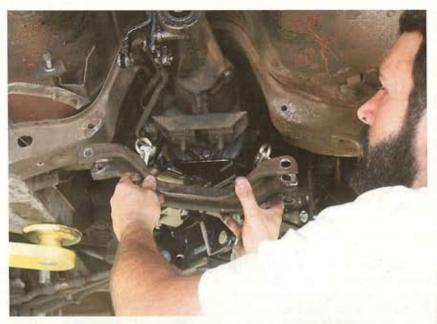
Modern Driveline's owner Bruce Couture came to our facility to perform the installation personally. He begins by removing the driveshaft and exhaust system. Here, the original T-10 gearbox is supported by a transmission jack while Couture removes the stock crossmember.
