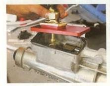
We've already removed the shifter that was supplied with the transmission, and here the Slick Stik unit is shown being installed in place of the original. We didn't use a gasket but rather a carefully applied bead of silicone sealer.
