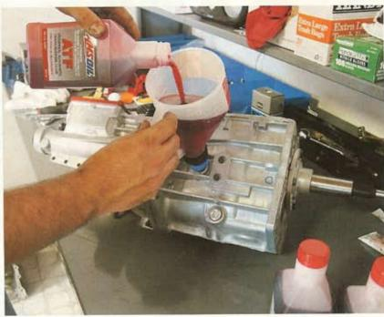
It's much easier to fill the transmission before it's installed, and the Amsoil automatic transmission fluid is included with the kit. Unlike a Top-Loader or a T-10, the World Class T-5 gearbox must use automatic transmission fluid. Regular-weight gear oil will ruin a T-5 because the viscosity is too high to allow cold circulation to needle bearings and other small moving parts.
