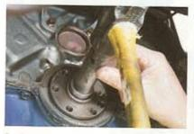
Back underneath the car, it's time to install the new pilot bearing into the crank. Unlike the original bushing, this part is a true bearing that uses needle bearings to support the transmission input shaft. Care must be used installing the bearing because it can be easily damaged.
