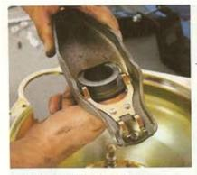
Install the release bearing onto the new clutch fork. Before the fork is installed into the bellhousing, the ball stud will receive a small coating of heavy grease. Don't use too much as you don't want excess grease getting into the clutch.
