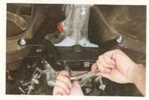
Because we were so careful installing the clutch, the transmission seated up against the bellhousing without a struggle. Here, the conversion crossmember goes into place. It's a perfect, no-hassle fit.
