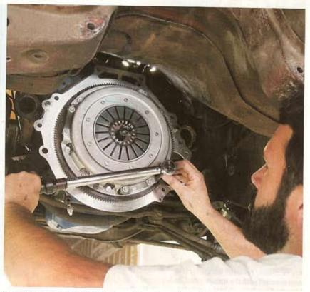
We made sure the alignment tool wasn't drooping when we began to tighten down the pressure plate fasteners. We torqued down the pressure-plate fasteners to the prescribed value, which is 25 ft-lb. The torque wrench was also used when installing the flywheel.
