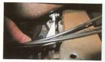
The adapter is bolted in place to the upper end of the pedal arm. The cable end is equipped with an eye that attaches to the adapter at the top using a pin and cotter key.
