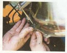
The cable casing is anchored to the bellhousing with a C-clip. At the top of the photo, the threaded end of the cable shows, and this is where any clutch adjustment takes place. Once the correct adjustment is reached, a jamb nut will be installed to lock the setting into place.
