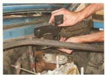
The cable support plate is installed. Determine the correct orientation by lining it up with the master-cylinder bolt holes. With the plate in the correct position, mark the firewall where the clutch cable will pass through. We used a hammer and a center punch to dimple the spot.
