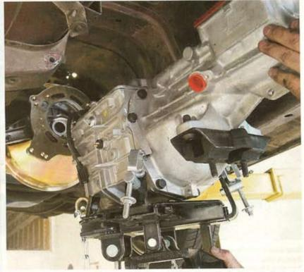
It's the moment of truth as the new gearbox is carefully balanced on the transmission jack. The transmission is raised and moved forward toward the bellhousing in small increments. We would say that from a safety standpoint the transmission is too heavy to do this step by hand, although we've seen it done many times.
