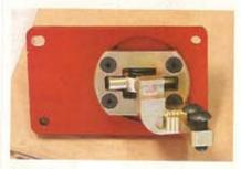
Although the new transmission comes with a shifter, we wanted to upgrade to this billet Slick Stik unit (PN MD-82-303-034103). This shifter moves the lever rearward by 1 inch, thus allowing installation without cutting the floor. This shifter is much stronger than the OE part and offers smoother shifting and a shorter throw, at a price of \$250.
