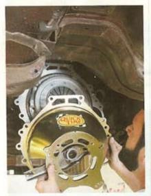
We're moving right along as the prepared bellhousing is installed onto the back of the engine. The QT part looks cool and adds safety with its SFI rating.
