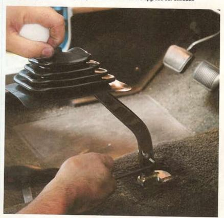
In the interior, two fasteners are used to install the shift handle. The boot will be secured to the floor with four small sheetmetal screws. The Slick Stik shifter clears the hole so nicely that we didn't need to enlarge the opening. The downside of not enlarging the opening is that the shifter can't be removed without dropping the transmission. Now to try out the 405 again.
