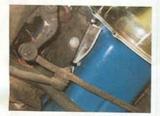
The heat-jacketed clutch cable housing is secured with an Adel clamp to one of the oil pan bolts on its way to the bellhousing. We're well clear of exhaust heat or any moving parts.
