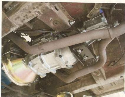
With our exhaust back in position, we've completed the gearbox installation. The next step is to reinstall the driveshaft, which we had shortened by 1 inch. While the shaft was out of the car, we also installed new U-joints. Everything fit perfectly, and the crossmember looks as though it will allow plenty of clearance when we upgrade our exhaust.
