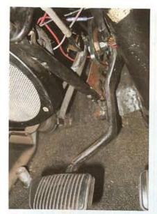
The original clutch linkage used a pushing movement with the pushrod attached to the pedal arm below the fulcrum. Since the new cable setup requires a pulling motion, the cable must attach to the pedal arm above the fulcrum. Looking at the pedal from below, it's possible to see how the adapting bracket is bolted to the side of the factory pedal arm using one fastener.
