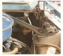
This is what the cable installation looks like with the plate installed behind the master cylinder. This is a durable arrangement because the steel used in making the cable support plate is of a much heavier gauge than the stamped steel used to make the vehicle firewall. The cable assembly is long enough so that the curve going back toward the bellhousing is a gentle one.
