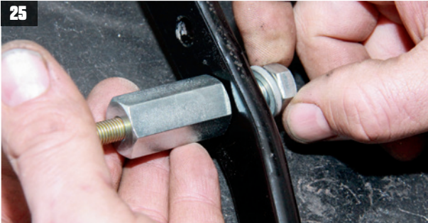
The Modern Driveline hydraulic clutch master cylinder pushrod connection is bolted to the stock Chevrolet clutch pedal.
