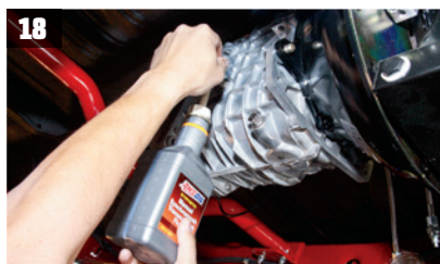
AMSOIL Manual Synchronesh Transmission Fluid is pumped into the TKO-600 until it reaches the bottom of the filler port, about 2.75 quarts.
