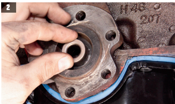
2 First up was installing the fresh pilot bushing included in the kit for the TKO install.
