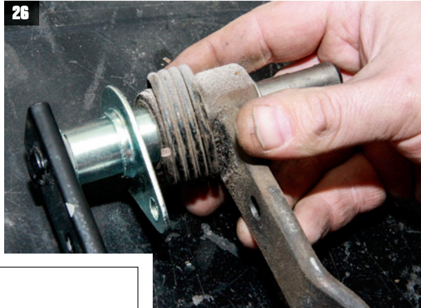
Modern Driveline suggests removing the clutch pedal helper spring because it will not be needed.
