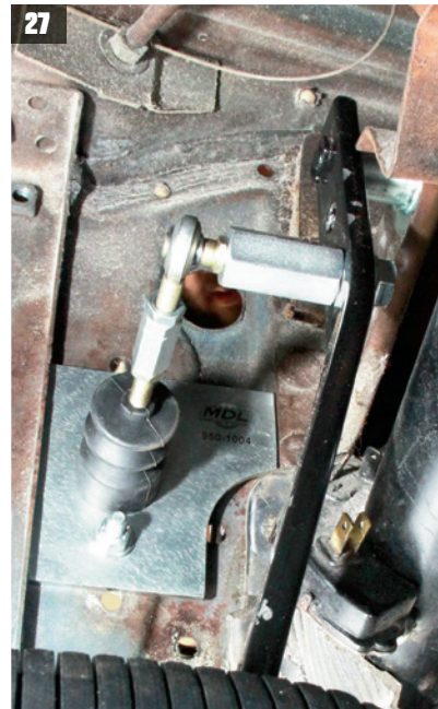
Here you can see how the Modern Driveline firewall plate is used to properly locate the clutch master through the firewall.
