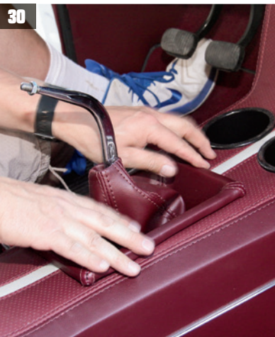
30 The TMI custom console is installed next along with the TMI boot. In all, we spent a full two days on the install. Modern Driveline offers a wide variety of five- and six-speed transmission conversion packages, including stock replacement bellhousings and performance shifters.
