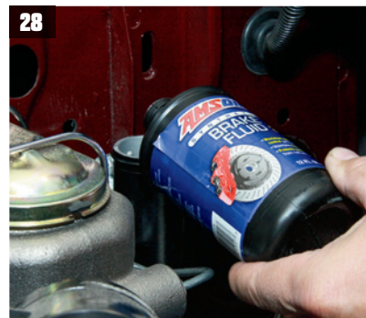
AMSOIL Synthetic Brake Fluid is added to the Modern Driveline clutch master cylinder for bleeding. A good DOT 3 fluid is recommended.
