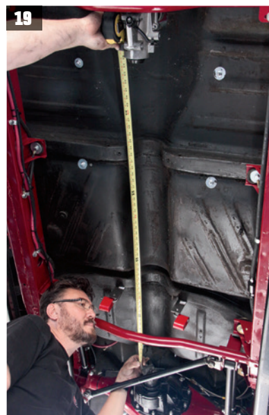
Here's the Modern Driveline crossmember bolted into place with the TKO transmission secure. As you can see, there's plenty of room in the transmission tunnel.
