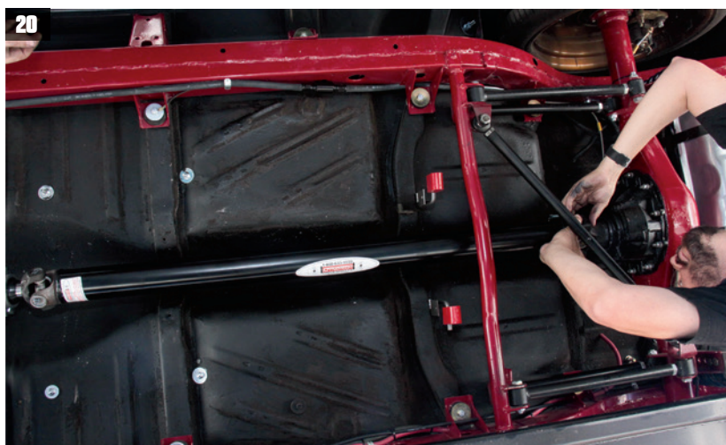
Our Dynotech driveshaft has arrived and is a perfect fit. Lube the forward slip yoke with transmission fluid to prevent seal damage.
