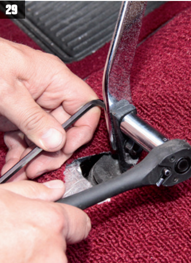
29 A hole for the shifter has already been cut in the transmission tunnel. The shifter handle is installed at this time along with the boot.
