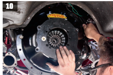
10 The Quick Time bellhousing is installed next, securing all of the bolts at the engine block. The Quick Time housing is SFI rated, which is a huge bonus in the highly unlikely event of a catastrophic failure.
