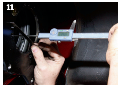
11 The clutch diaphragm depth is checked here as shown to determine the release bearing depth adjustment.
