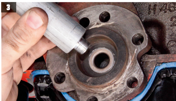
3 The pilot bushing or bearing can be driven in with an appropriately sized deep-well socket or a driver like this one, which drives the bushing in without damage.
