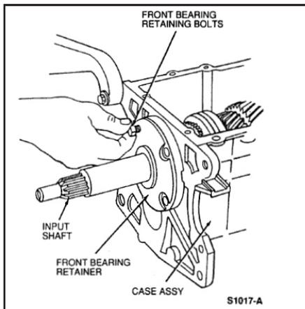
3. Remove front bearing retainer.
