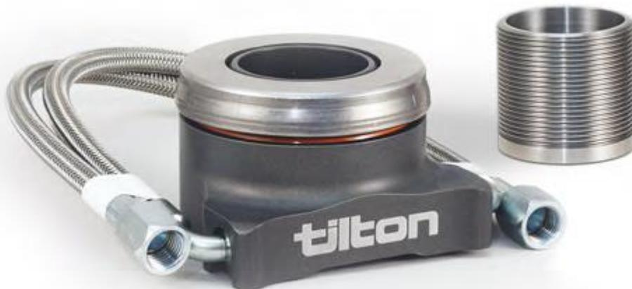
The Tilton hydraulic release bearing assembly is self-adjusting once proper set-height has been accomplished. The bearing will always be in contact with the pressure plate fingers, but not under constant load or preloaded. When the clutch pedal is released the bearing will only return to the point of contact. There will not be a “gap” between the bearing and pressure plate fingers.
