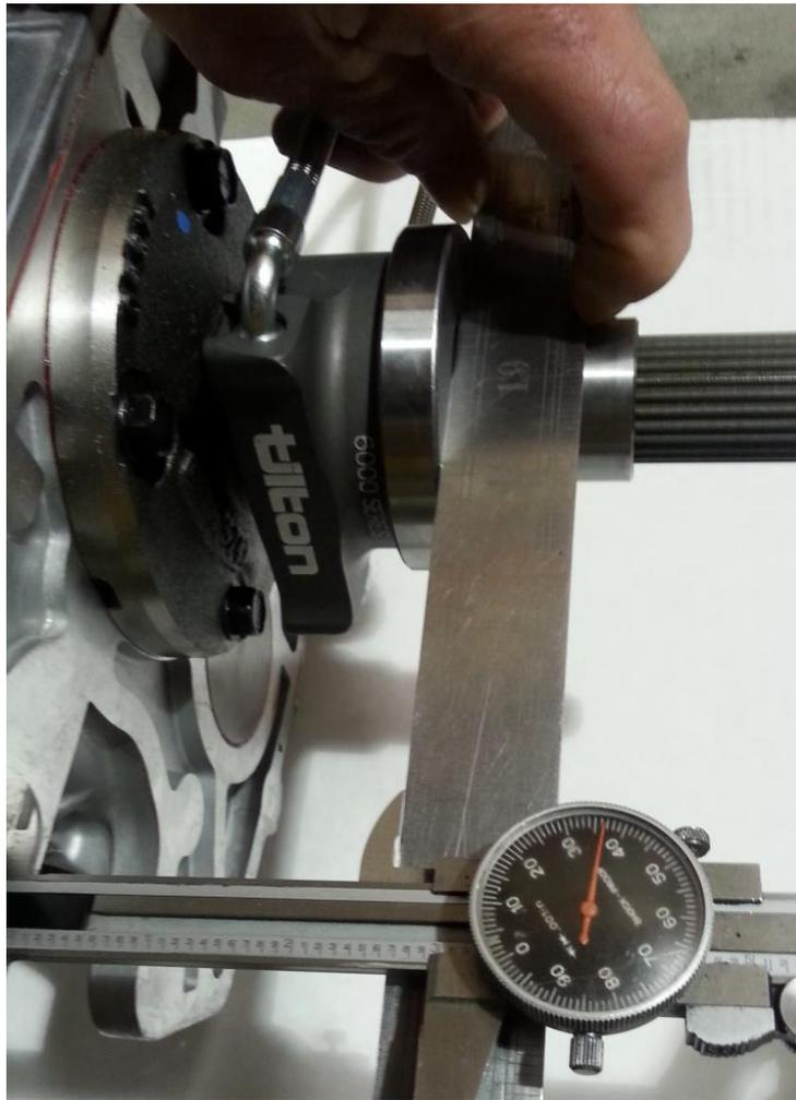
Diagram 2 – Dimension A \_\_\_\_\_ - .125 = \_\_\_\_\_ Dimension B
