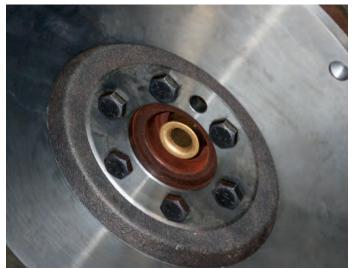
7 The bushing is inserted and centered for installation.
