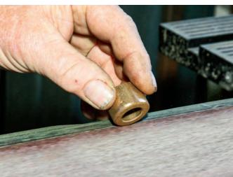
The clutch pilot bushing is dressed on a sanding belt to give it a taper for easy installation.
