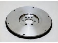
MDL inventories a wide variety of flywheels in steel and aluminum for all Chevrolet applications. Begin your alignment process with a new flywheel for pinpoint accuracy. Opt for ARP flywheel and clutch bolts while you're in there using a thread locker before torqueing the bolts in a crisscross fashion to Chevrolet's specifications. Tighten bolts in one-third values, then recheck your work.
