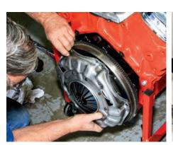
Twith the alignment tool and disc properly centered, install the Superior pressure plate. Bolts should be snugged in a crisscross fashion for uniform installation, then torqued crisscross in thirds. Then, check torque around the perimeter a final time.
