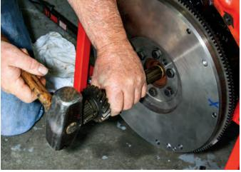
A transmission input shaft makes a nice clutch pilot bushing driver. You can even use it as a clutch alignment tool. The bushing is driven until seated in the crank. It is suggested you spend the money and opt for a clutch pilot bearing, which delivers smooth operation.
