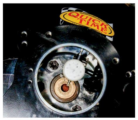
Set up your dial indicator with the pin just touching the inside diameter of the bell opening and set the needle at zero. The dial indicator bracket should be attached to the flywheel. Dial indicators are available from Harbor Freight, or any tool store.
