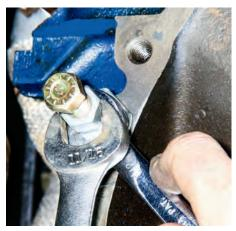
14 When old alignment pins won't come out by conventional means we have to try an unconventional approach. Bruce encountered stubborn alignment pins that would not come out. He welded a bolt to the pin and drew it out with a nut as shown.
