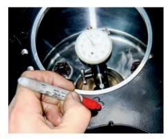
Note your findings on the bell with a marker each time you make a full pass. If your numbers are inconsistent check the dial mounting and setup.
