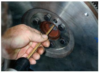
The clutch pilot bushing pocket at the crank flange should be dressed with 180-grit paper as shown and cleaned up for the pilot bushing or bearing.
