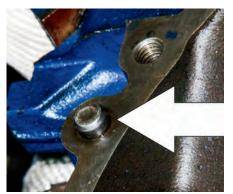
13 Engine blocks are fitted with bell-housing alignment pins (see arrow), which ensure bell alignment with the block. Sometimes these pins are too short or misaligned and must be replaced.
