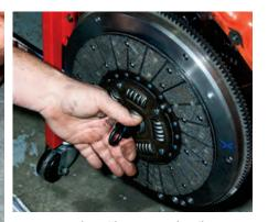
16 We're installing a Superior diaphragm clutch from MDL on a bigblock Chevy. Spot-on bell alignment must be followed by accurate clutch, disc, and pressure plate alignment. You can use the clutch alignment tool MDL provides or a transmission input shaft. Pressure plate and flywheel contact surfaces must be hospital clean, which can be accomplished with brake cleaner.
