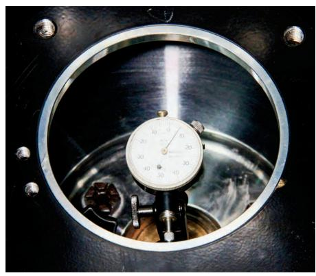
Turn the flywheel/crank slowly for 360 degrees and closely watch the needle. Needle movement should be 0.010-inch or under. It's a good idea to repeat this procedure to see if the gauge repeats these numbers. If there's any doubt, repeat the procedure until you are positive of your findings.
