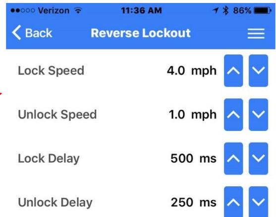
There is really no reason to change any settings on the Reverse Lockout Solenoid. The default settings are recommended, which will allow the shifter to easily go into reverse from 0 – 4 mph and will have the spring detent to make going into reverse difficult above 5 mph.
