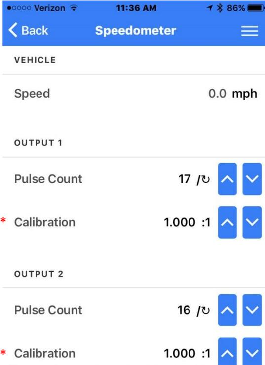
Next select the Speedometer menu. This will allow you to adjust the pulse signal output to match your specific requirements for your speedometer. \* This is specified by your gauge manufacture and should confirm with them when changing this setting.
