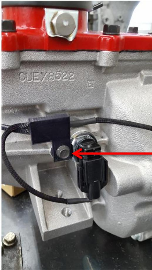
The epoxy sealed control module should be attached to the transmission using the bolt that fastens the speed sensor clamp.
