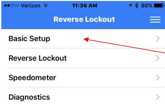
Once you have the phone connected to the All-In-One it will take you to this Main Menu screen where you can select which feature you need to adjust. Start with the Basic Setup menu first.
