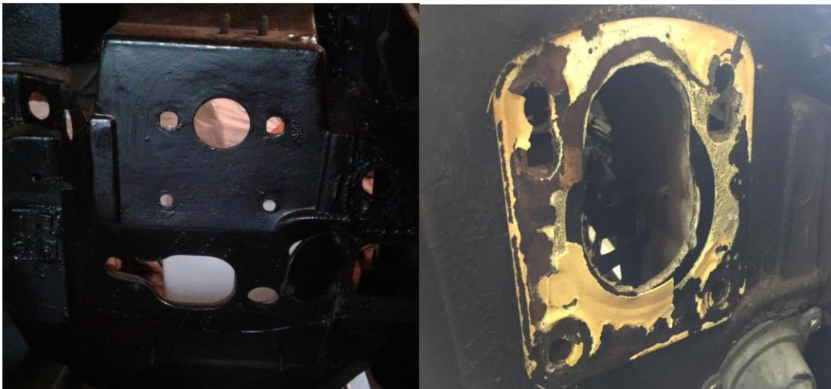
3.2 Prefit the firewall plate to the firewall. Verify the hole pattern aligns and temporarily bolt in place using existing vehicle hardware.
