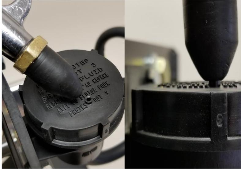
2.25.3 Since the reservoir is small, the bleed screw should only be open for about 5 seconds. You will see a solid stream of fluid come out, followed by air bubbles, followed by another solid stream of fluid. Immediately close the bleed screw when you see the second solid stream of fluid to prevent draining the reservoir.
