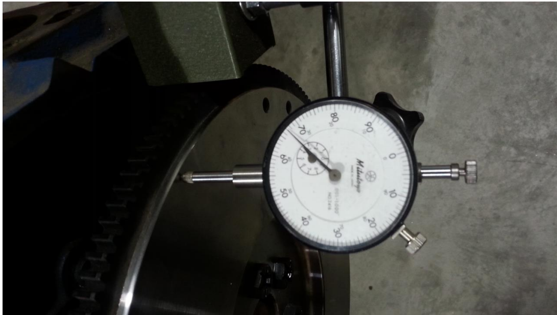
Shown is the Flywheel Run-out check. Mount the magnetic base to the block and dial indicate the flywheel to check flywheel run-out.
