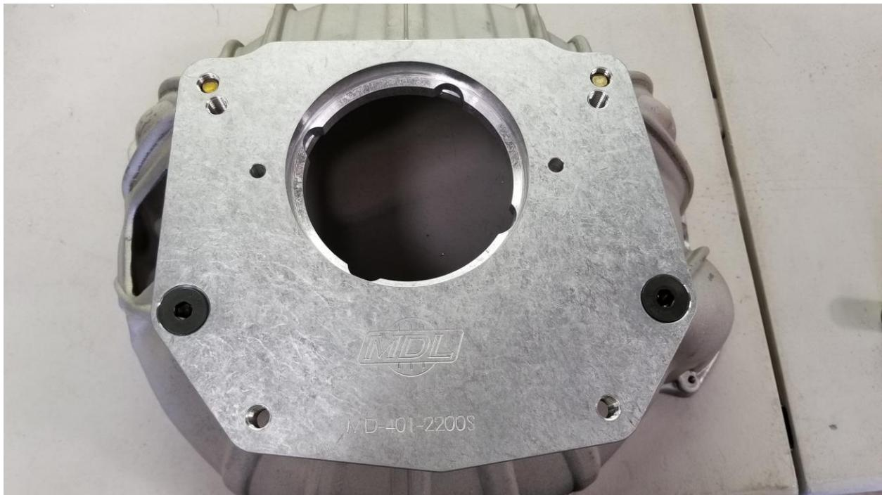
Install (4) 7/16"-14 supplied fasteners for transmission and torque to 19 ft/lbs (dry) or 15 ft/lbs with anti-seize compound applied.
