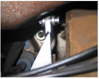
For installation from stock linkage to clutch cable, install 1 ½" body plug into the clutch rod hole.
