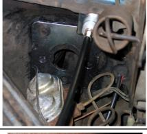
Thread the ¼" cable end into the clevis until the end is flush with the clevis. The end of the cable should not protrude into clevis opening.
