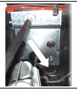
Clearance the clutch pedal bracket. The assistant spring tab must be removed at the yellow line.
