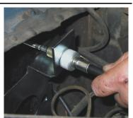
Install the fasteners for the brake master cylinder or brake booster. Center the plate to ensure the cable will not drag across the firewall.
