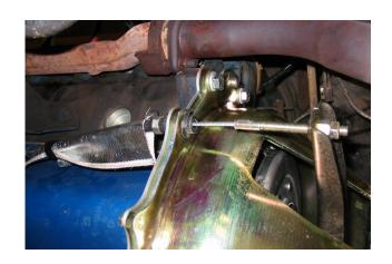
Adjust cable travel at clutch fork. Fine adjustment of the cable can be done at the firewall by turning the adjuster on the support plate. Turning the nut clockwise will tighten the cable. There should be minimal slack in the cable when properly adjusted.
