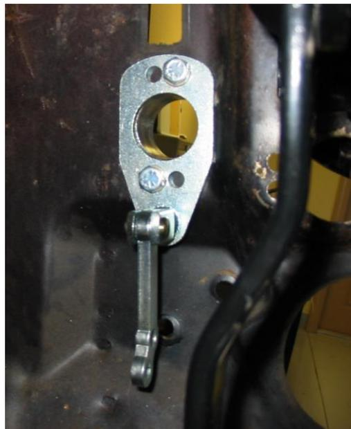
3.6 Remove master cylinder spacer block. Touch-up and deburr firewall as required.
