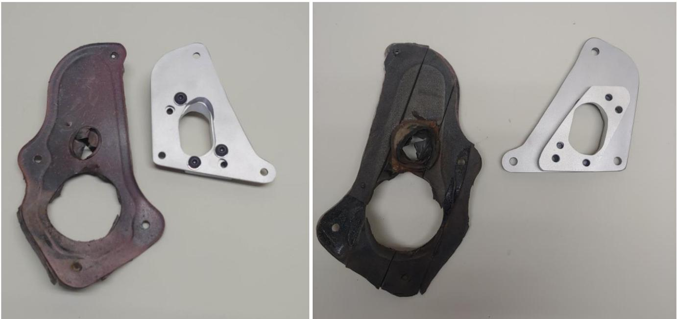
**Shown is the original steering column plate compared to the new hydraulic clutch master cylinder block and plate.**
