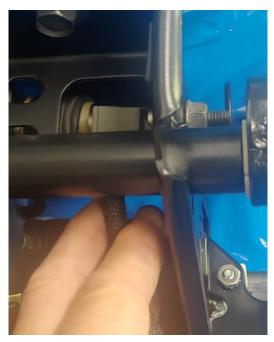
3.11 Re-attach the steering column shaft to the knuckle joint. Remove the temporarily installed bolt form the knuckle joint using a 10mm socket. Verify and restore orientation of the steering wheel and tires if either of these has moved. Insert the inner collapsible steering shaft into the knuckle joint and re-install bolt and tighten 18-22 ft/lbs.
