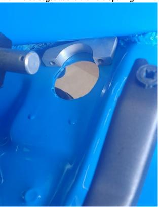
Shown are the insulation liner and excess sealant removed.
