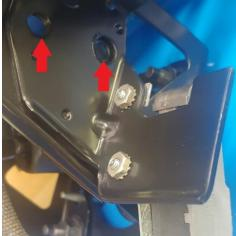
3.5 Position the magnetic nut-plate to the pedal hangar as shown. Nut-plate should sit flat where the red arrows are in previous picture. Install supplied fasteners in both red arrow holes in below picture to align. Verify threads go into both holes at the same time. Carefully remove fasteners not to disturb nut-plate position.
