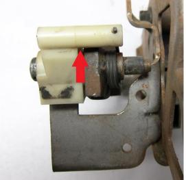
Use long skinny screwdriver to pry spring from arm. Cut plastic gear at red arrow.
