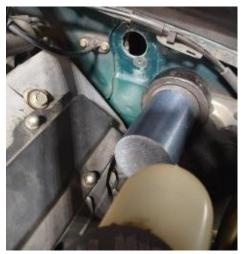
Cable installed, Cable removed, pedal linkage remains installed with all necessary parts removed.
