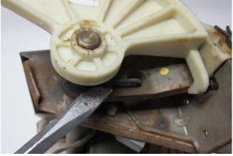
Use pliers or hook tool to remove clip. Push a screwdriver up between pedal arm and spring; it will spring loose and come off easily.
