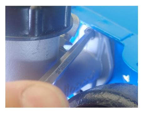
3.4 Transfer the removed cruise control switch parts to the new plate assembly and install. Carefully snug-up 5.5mm & 9mm fastener heads. The RED arrows will be where the magnetic nut plate gets positioned.
