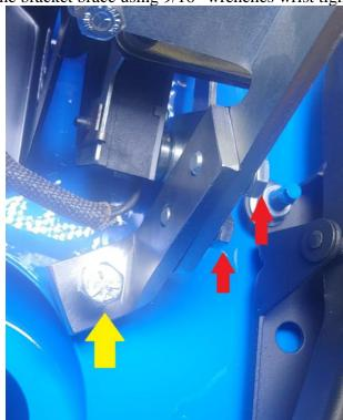
3.10 Using supplied zip-tie secure the cruise control cut-off switch harness inside the pedal hangar and route as shown.
