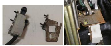
Shown is the Neutral Start Switch removed and the mounting bracket from under the dash.
