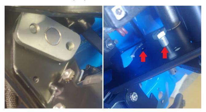
3.6 For this operation the clutch pedal pad will have to be held in the up position. Install 2 black nylatron bushings in the main bracket. Install the main bracket and ramp as an assembly into the vehicle and secure with hairpin clip. Swing the main bracket into position per the below picture series. Swing the ball-end on the m/c up and inboard to clear the ramp then allow the ball-end to settle into the ramp cup. Allow assembly to hang.
